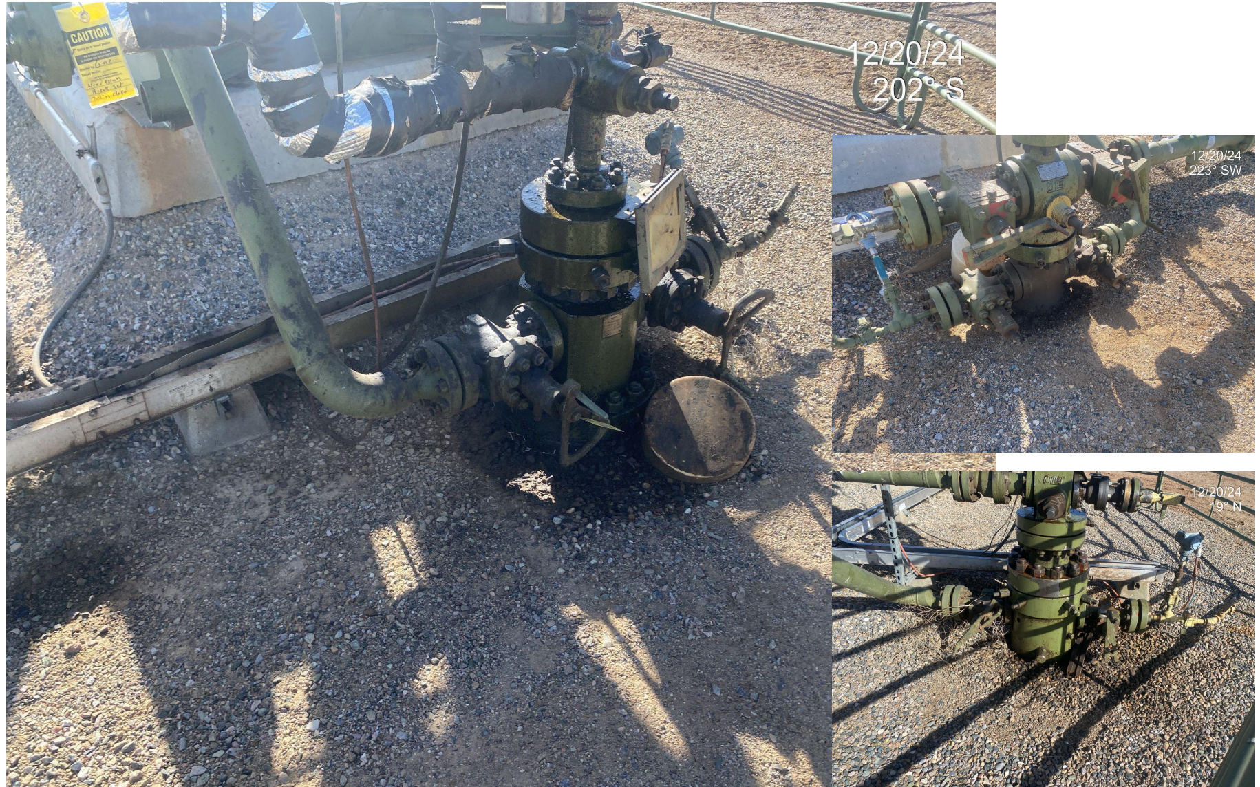
Photo 2. Impacted surface material observed at all three well heads on location.
