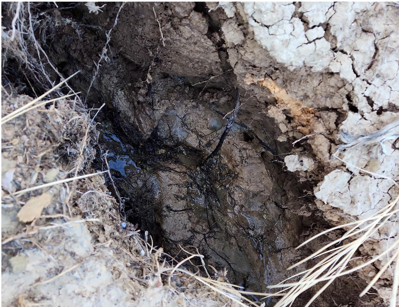
**Deep erosion channel cut by spilled fluids. Approximately 12-14 inches deep.**
