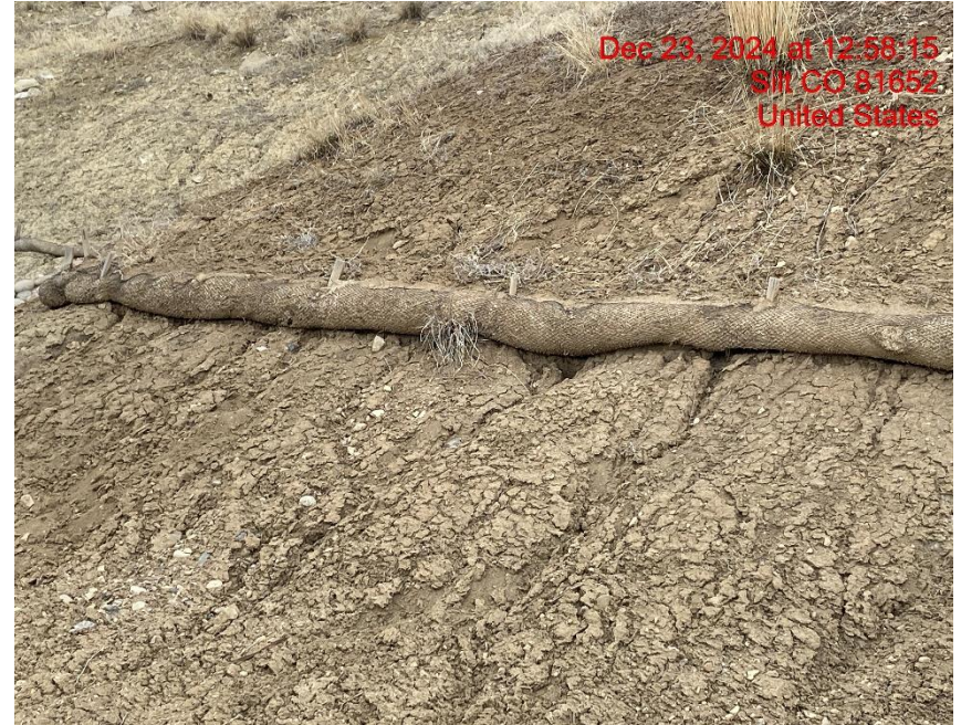
Rill Erosion Undercutting BMP – Photo #05562
