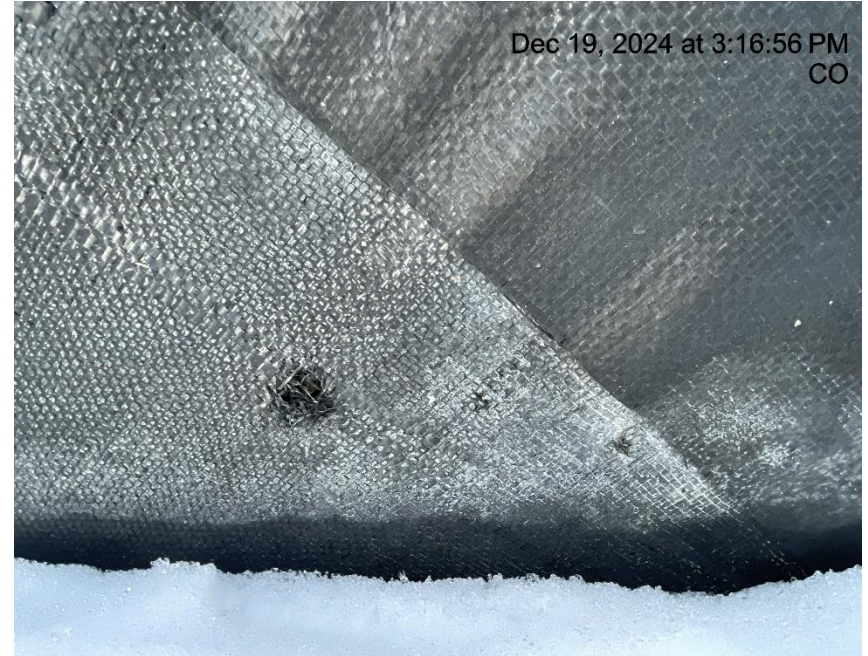
Photo # 4745 Hole in liner/liner needs maintenance
