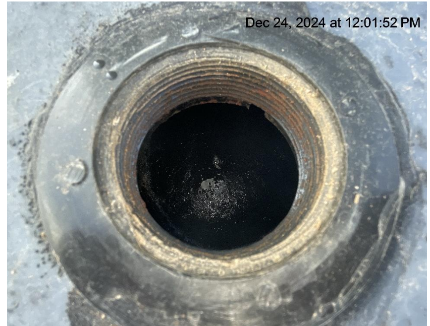
Photo # 5282 Failure to maintain chemical BMP - Chemical tank containment approximately 2/3 to 3/4 full of fluid/BMP insufficient to contain possible spill
