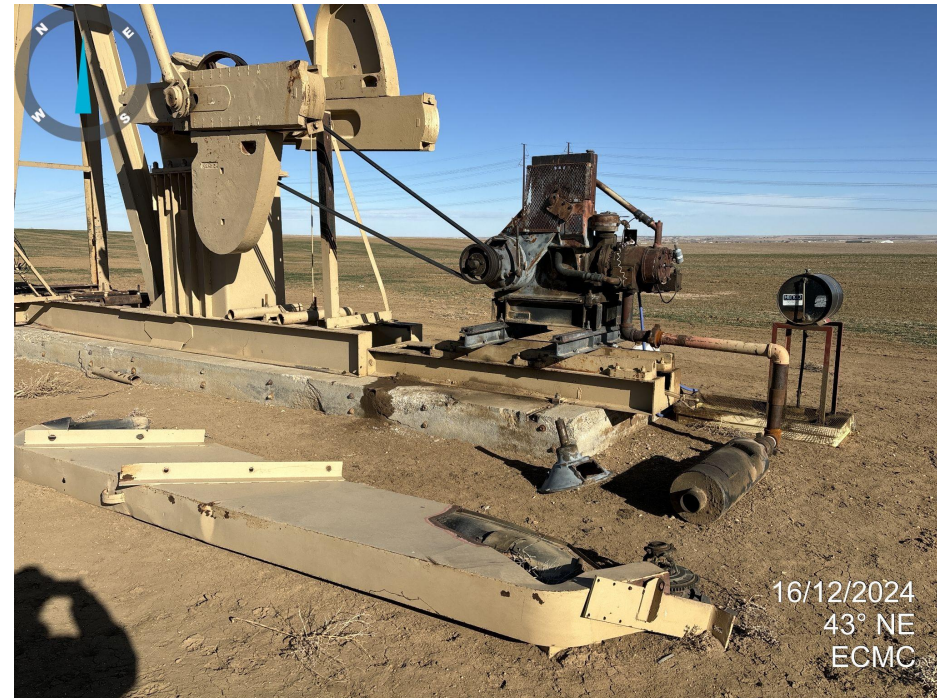
Photo 2. Pumpjack appears to be partially dismantled and unused equipment is left on site.
