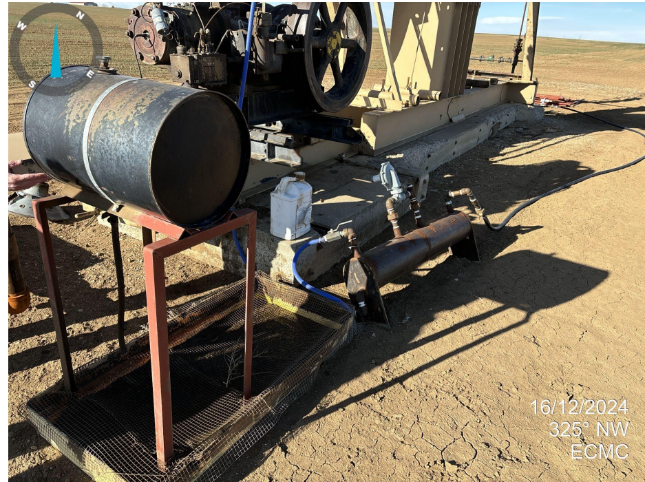
Photo 4. Barrel does not have label. Chemicals stored out of secondary containment.
