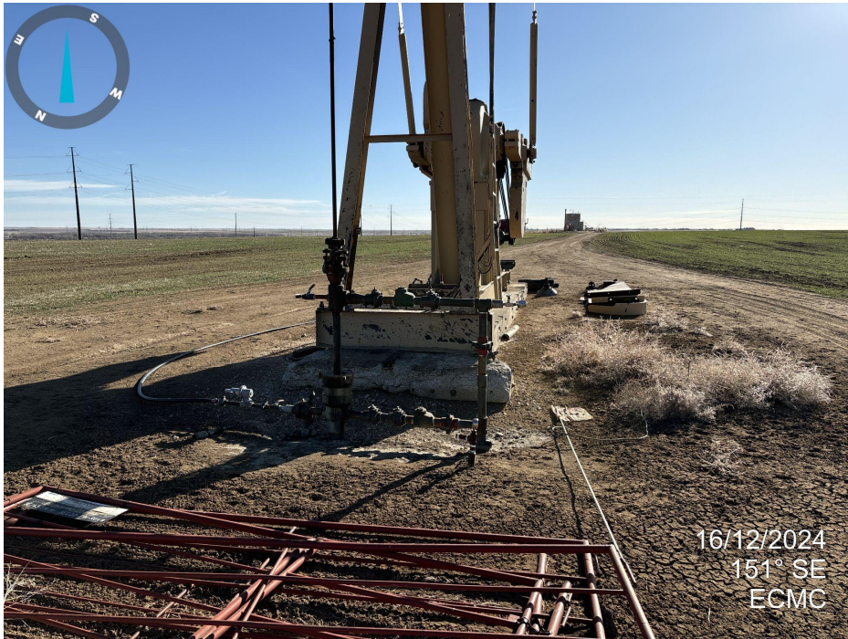
Photo 3. Fencing is not installed around pump. Undesirable annual plant species are present (Kochia).
