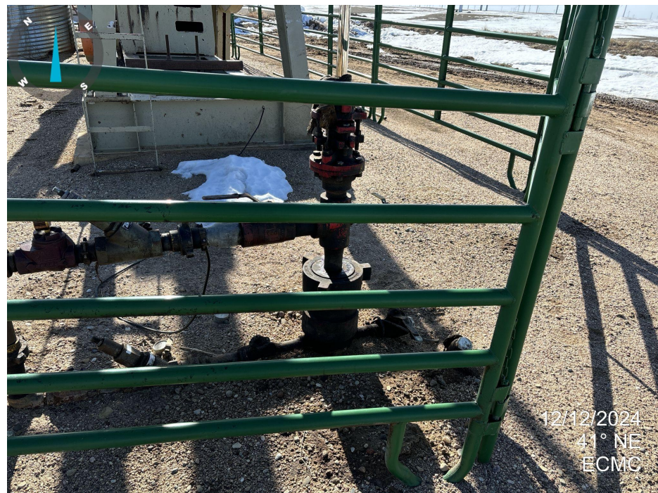
Photo 6. Stained soil around wellhead.
