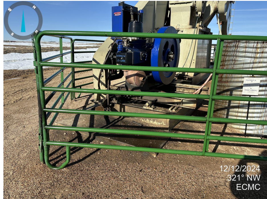
Photo 4. Soil staining possibly from oily exhaust/engine.
