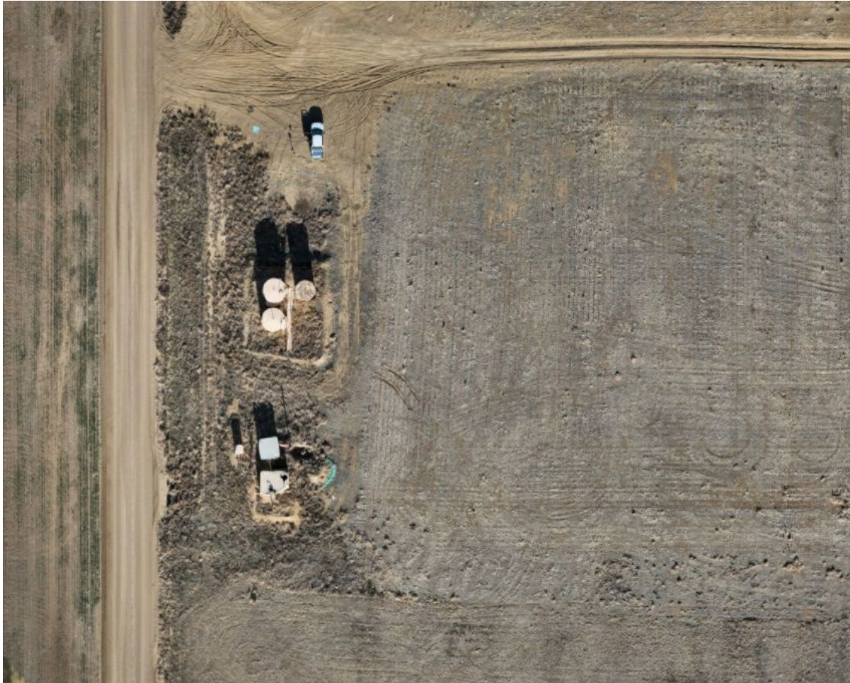
Photo 1. ECMC drone imagery taken on 12/18/2024. Overview of tank battery location. Imagery illustrates equipment has not been removed and an open excavation is present near the northern separator.
