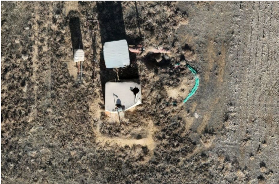
Photo 8. ECMC drone imagery taken 12/18/2024 of the excavation site. Stormwater BMPs are present around soil pile.
