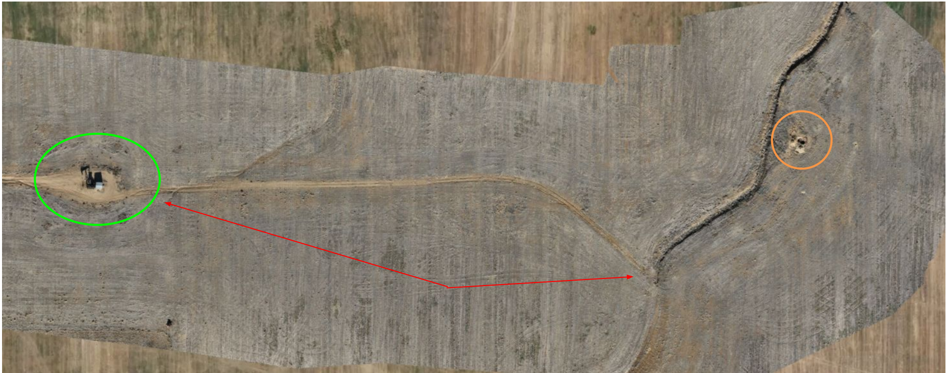
Photo 1. ECMC drone imagery taken on 12/18/2024. Overview of well location (orange) and access road (red arrows). Open excavation is present at wellsite, access road has not been reclaimed. Green circle = the active Doris #12-34 well (API # 123-10420).
