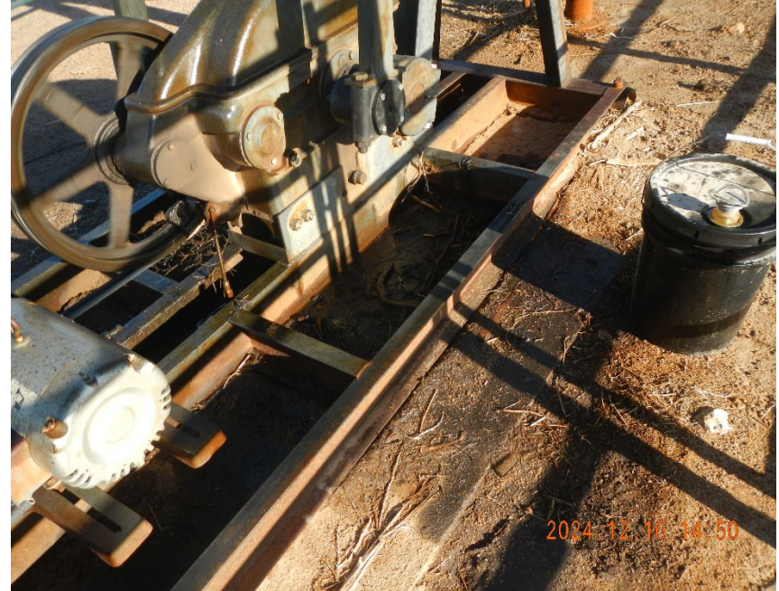
4. Lube oil on cement and soil at pumping unit gear box.
