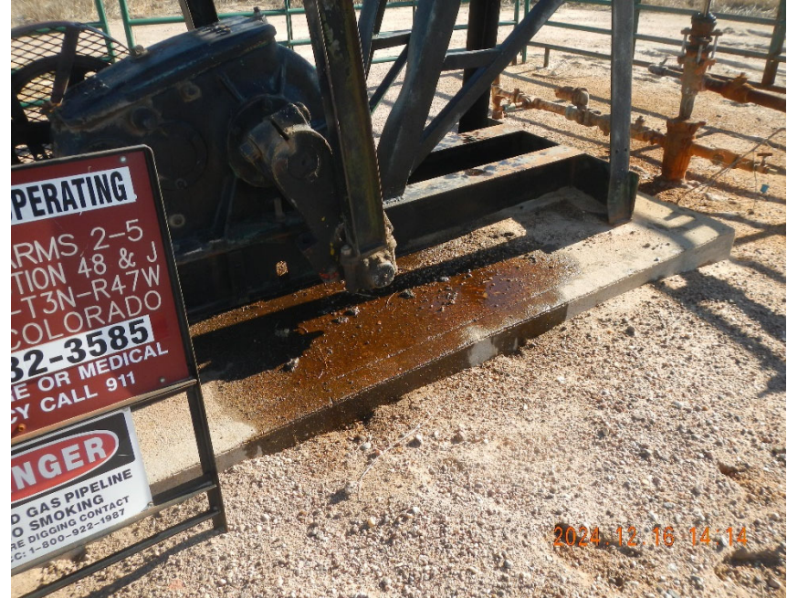
4. Additional view of oil leaking from gear box.
