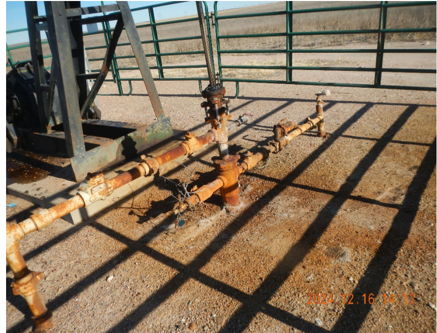
2. View of wellhead. Note staining around wellhead.
