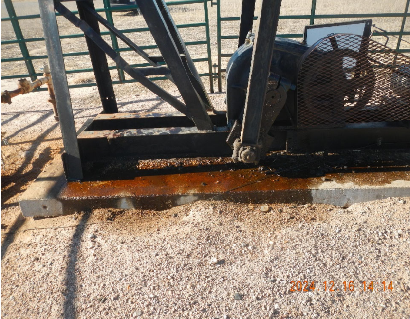
3. View of oil that has leaked from the gear box.
