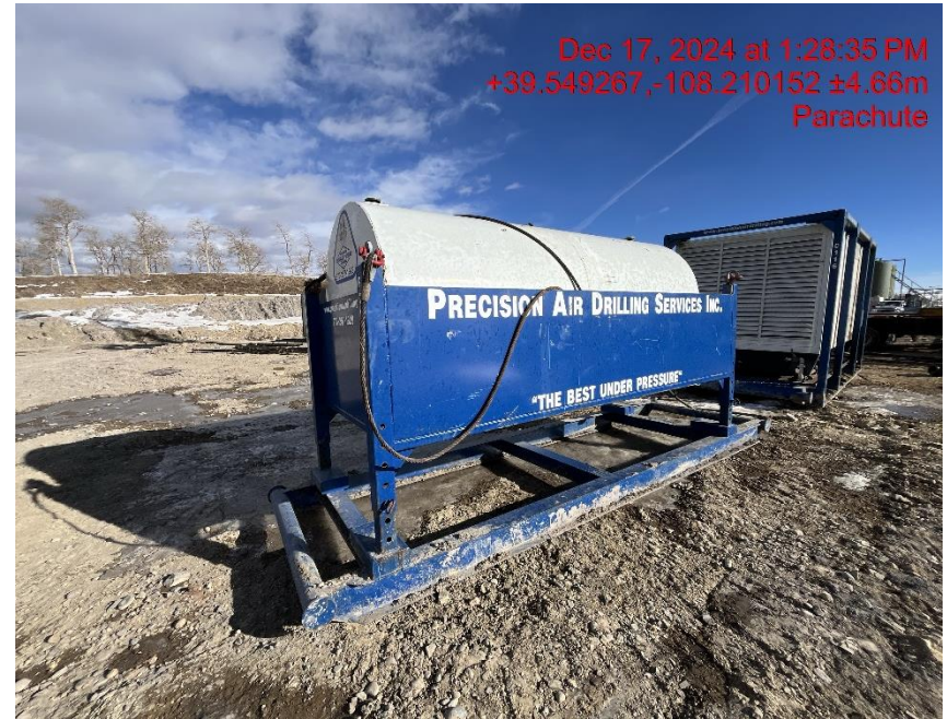
Photo # 1343 Tank lacks required information/does not comply with CECMC labeling rules
