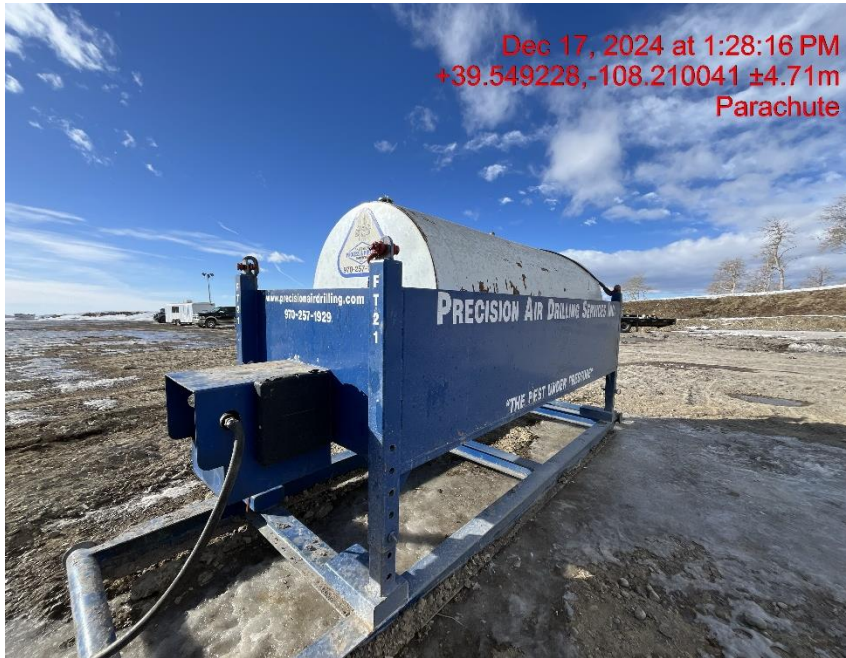
Photo # 1341 Tank lacks required information/does not comply with CECMC labeling rules
