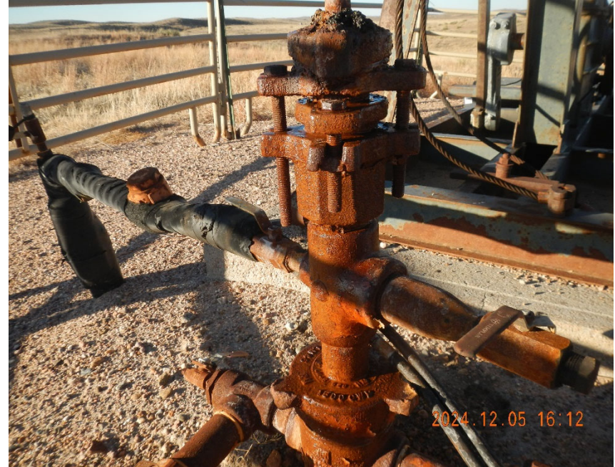
4. Closer view of wellhead tree.
