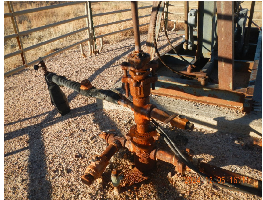
2. View of wellhead. Cap and area around base of wellhead is wet from produced water seeping at the packing.
