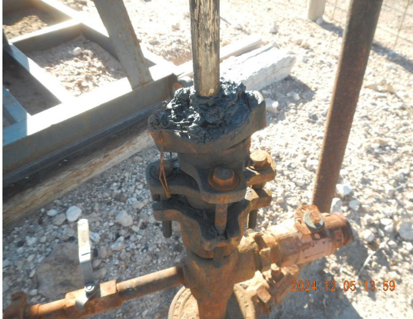
3. View of polish rod packing. Not leaking.
