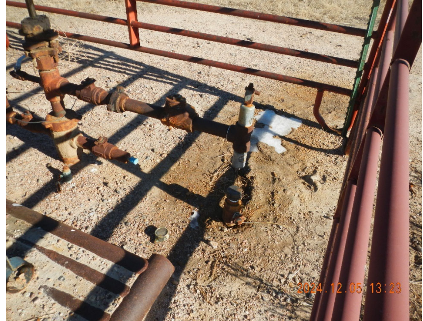
4. Additional view of wellhead showing water leg disconnected from wellhead.
