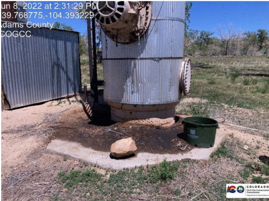
Photo 3. Photo from 06/09/2022 inspection (#699504016) illustrating stained soil at separator.
