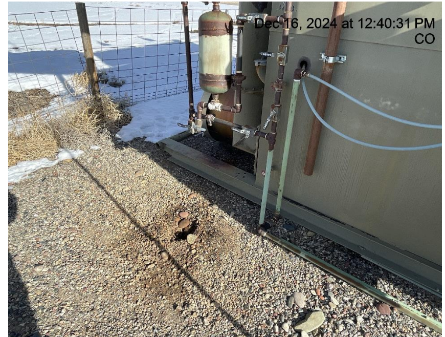
Photo # 3748 Staining near separator
