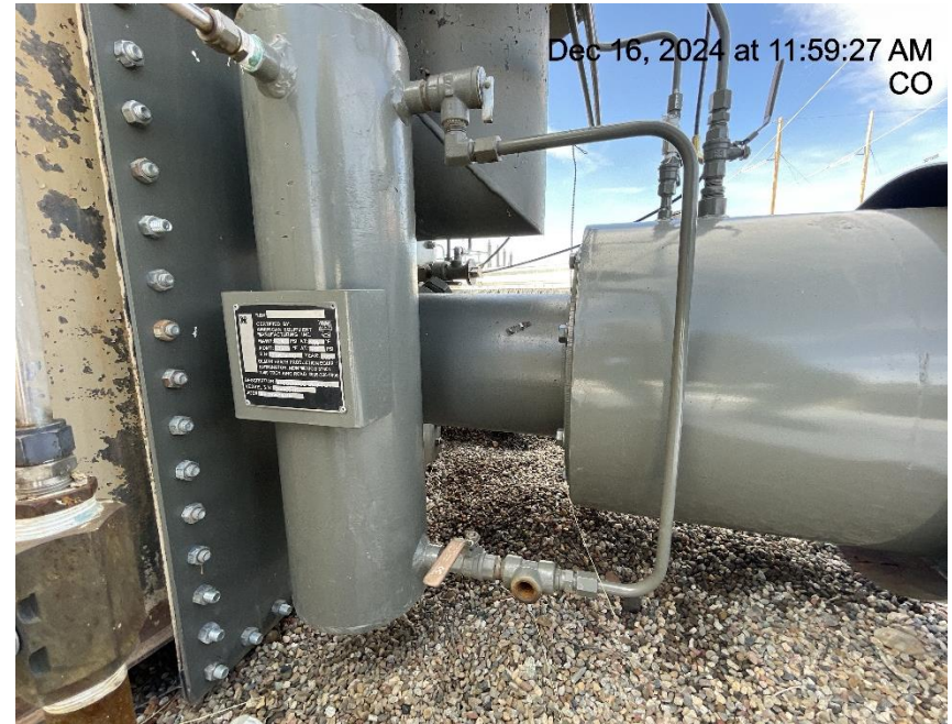
Photo # 3676 PRV vent line on tank burner does not comply with CECMC pressure safety device rules
