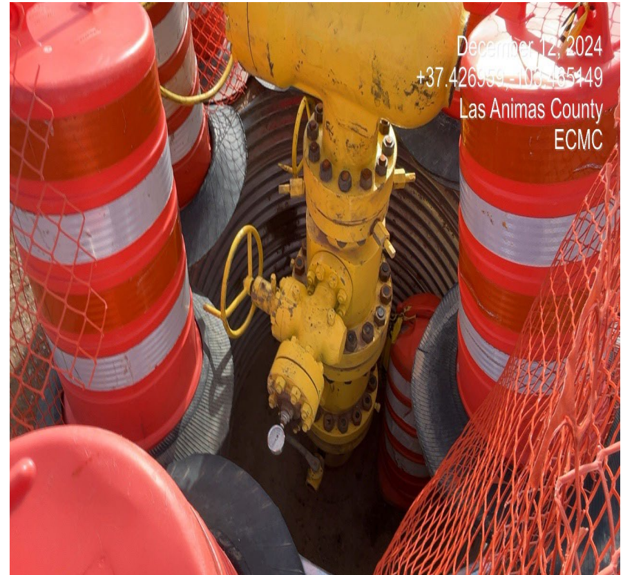
Photo 6. The open cellar at the wellhead does not have adequate wildlife protections..
