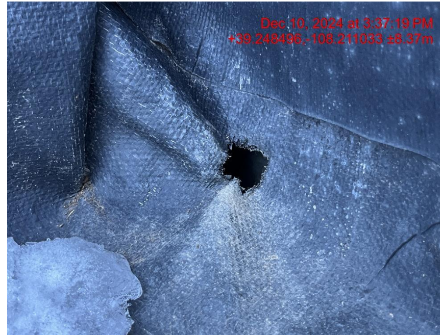
Photo # 0753 Hole in containment liner
