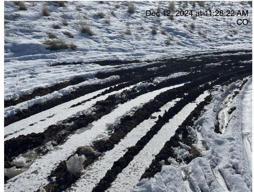
Photo # 3398 Lack of stabilization/compaction
