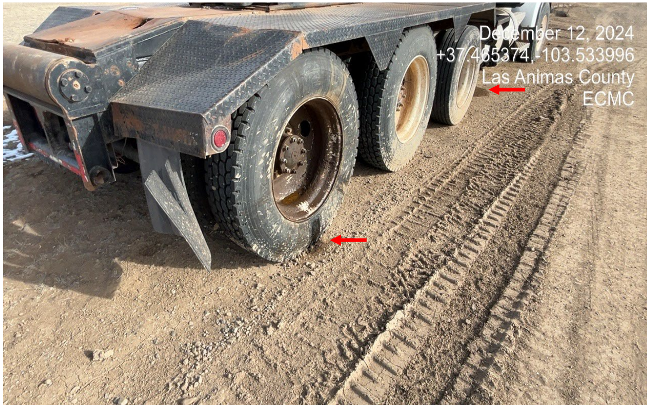
Photo 2. There is oil leaking from the wheel hub and stained soils that need to be cleaned up.
