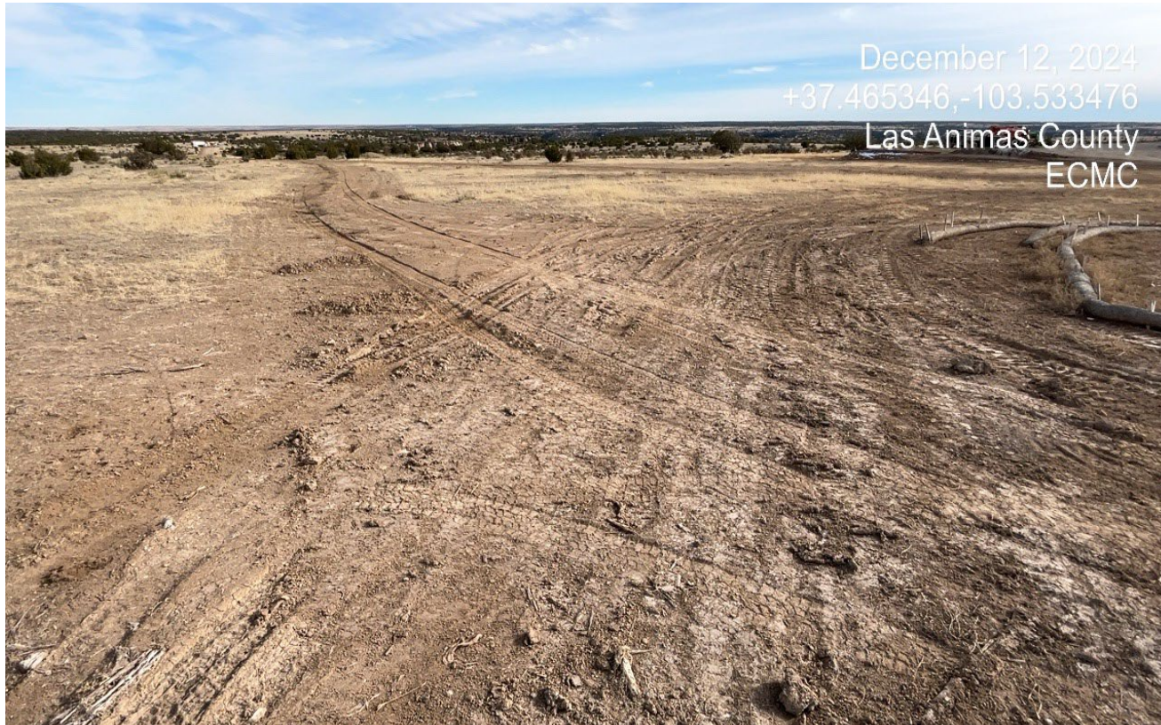
Photo 5. Facing south at the location. There are vehicle tracks along the flowline disturbance and vegetation is not establishing.
