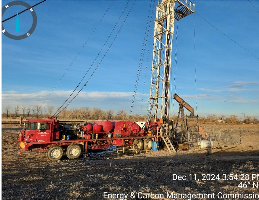
Photo 1 well head and equipment
