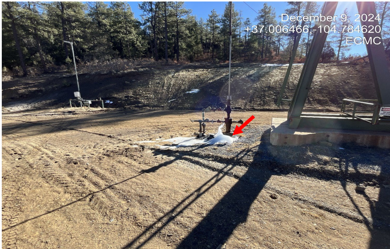
Photo 4. There is ice build up of a slight water leak at the wellhead.
