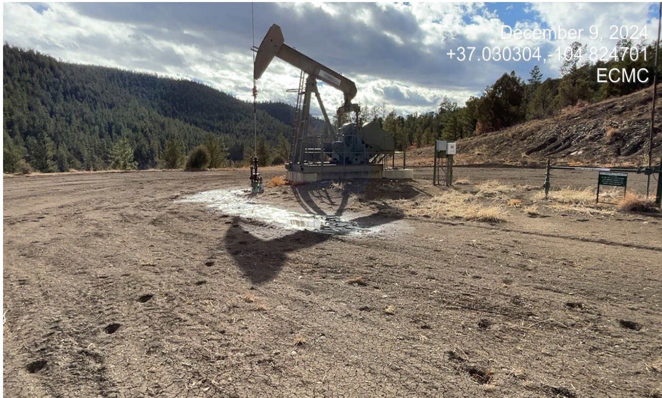
Photo 2. Facing toward the wellsite. There is a dripping water leak at the wellhead that needs to be controlled.
