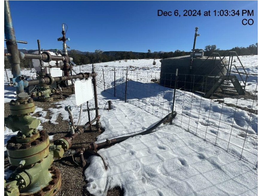
Photo # 2582 CIRCLE B LAND 14C-35-692 well bradenhead line connected to blowdown tank
