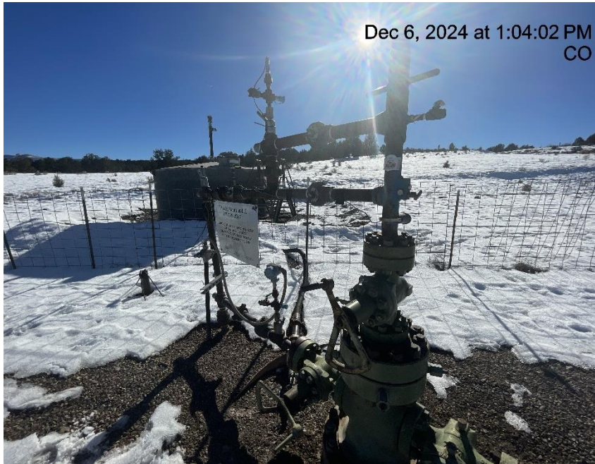
Photo # 2583 CIRCLE B LAND 14C-35-692 well bradenhead line connected to blowdown tank
