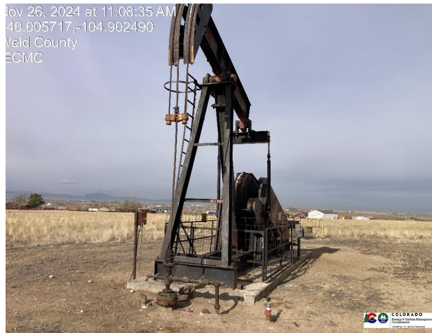
Pic 1 wellhead / pumpjack
