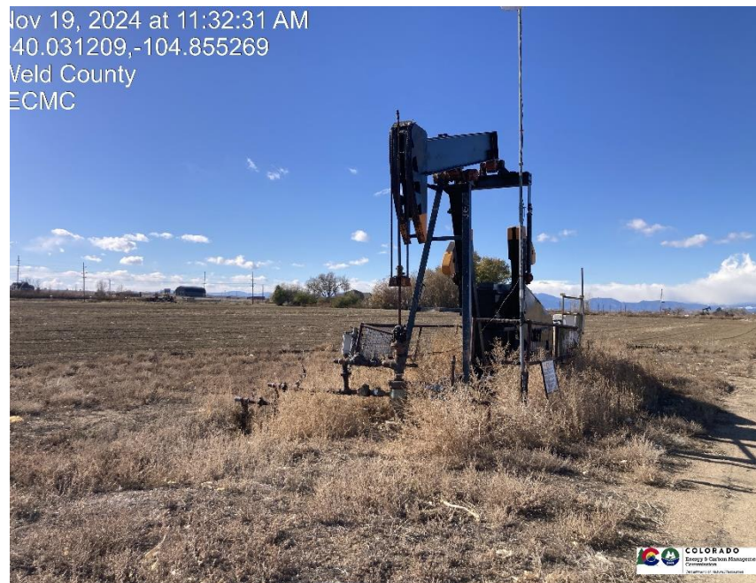
Pic 1 wellhead / pumpjack
