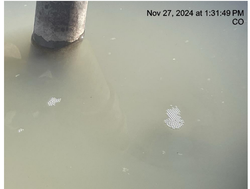
Photo # 1607 Mechanical Condition - possible bradenhead leak on the RMV 33-20 well
