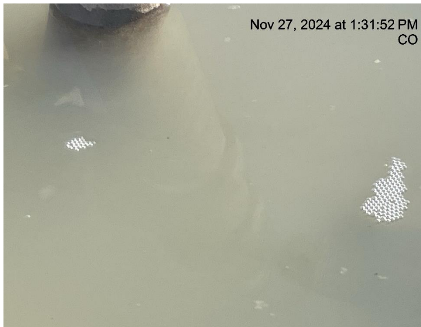
Photo # 1608 Mechanical Condition - possible bradenhead leak on the RMV 33-20 well
