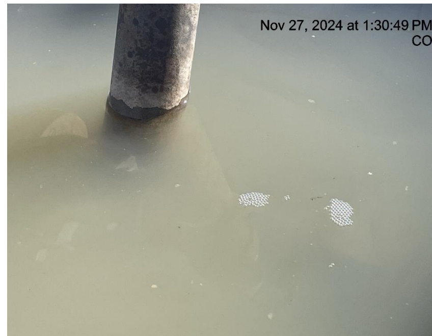
Photo # 1605 Mechanical Condition - possible bradenhead leak on the RMV 33-20 well
