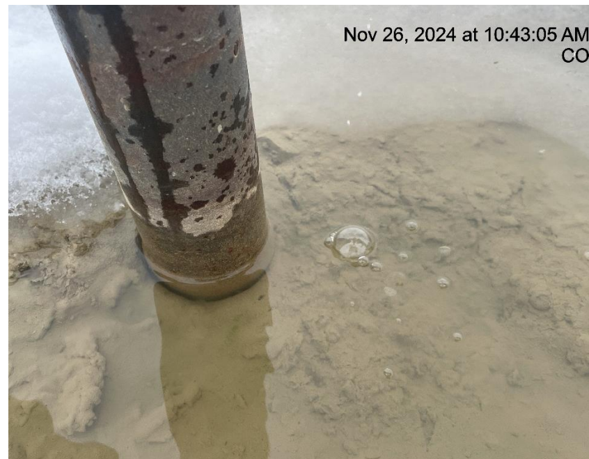
Photo # 1348 Mechanical Condition - possible bradenhead leak on the RMV 33-20 well
