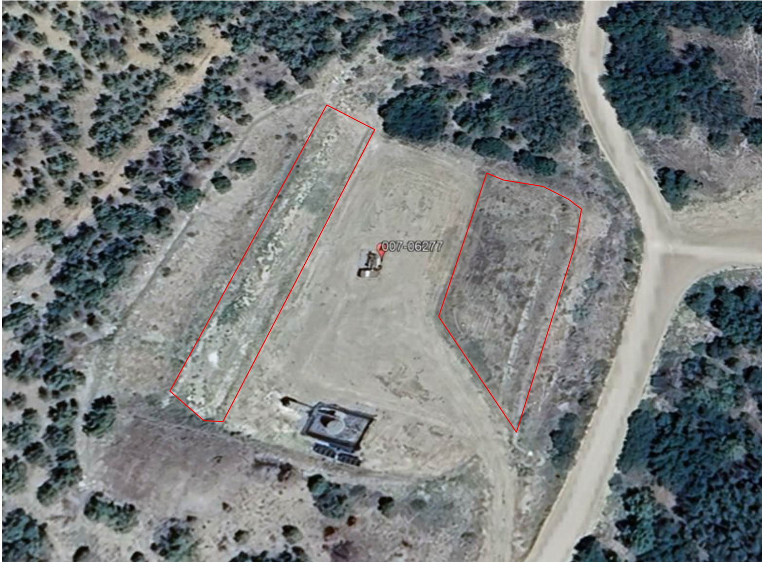
Photo 4. 2024 aerial imagery of areas on well pad which have not been reclaimed per 1003 requirements/standards.
