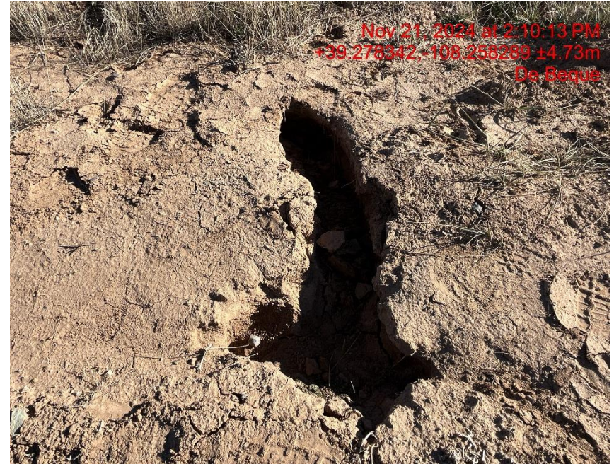
Photo # 9649 Subsidence in multiple areas on east side of location is also a wildlife/personnel safety hazard
