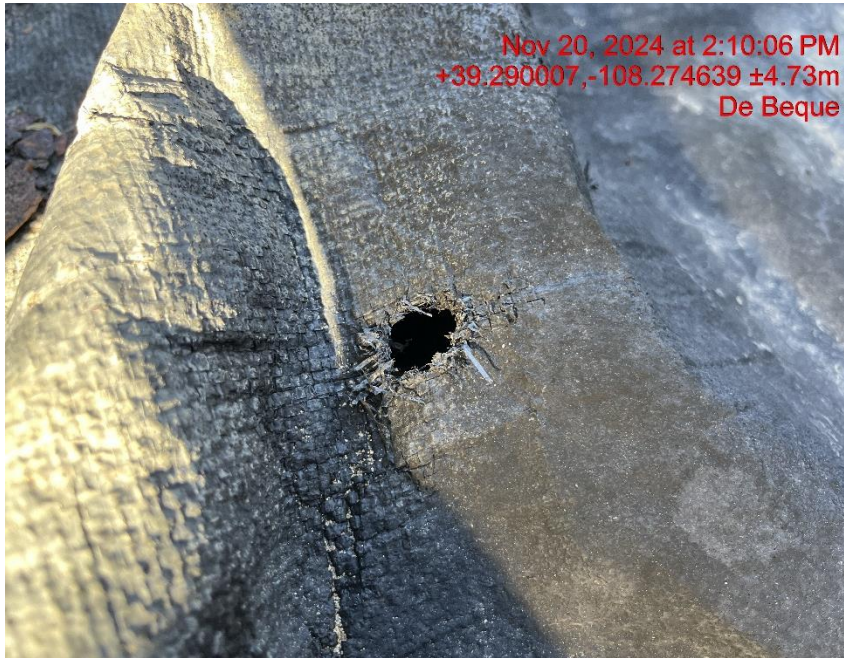
Photo # 9385 Multiple holes and tears in secondary containment liner/liner needs maintenance, also the liner is deteriorating and lacks integrity
