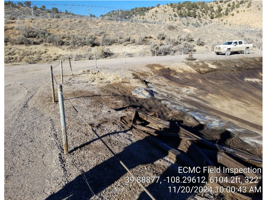
Photo #6 - Stained soil (E&P Waste) located on pit berm (2).
