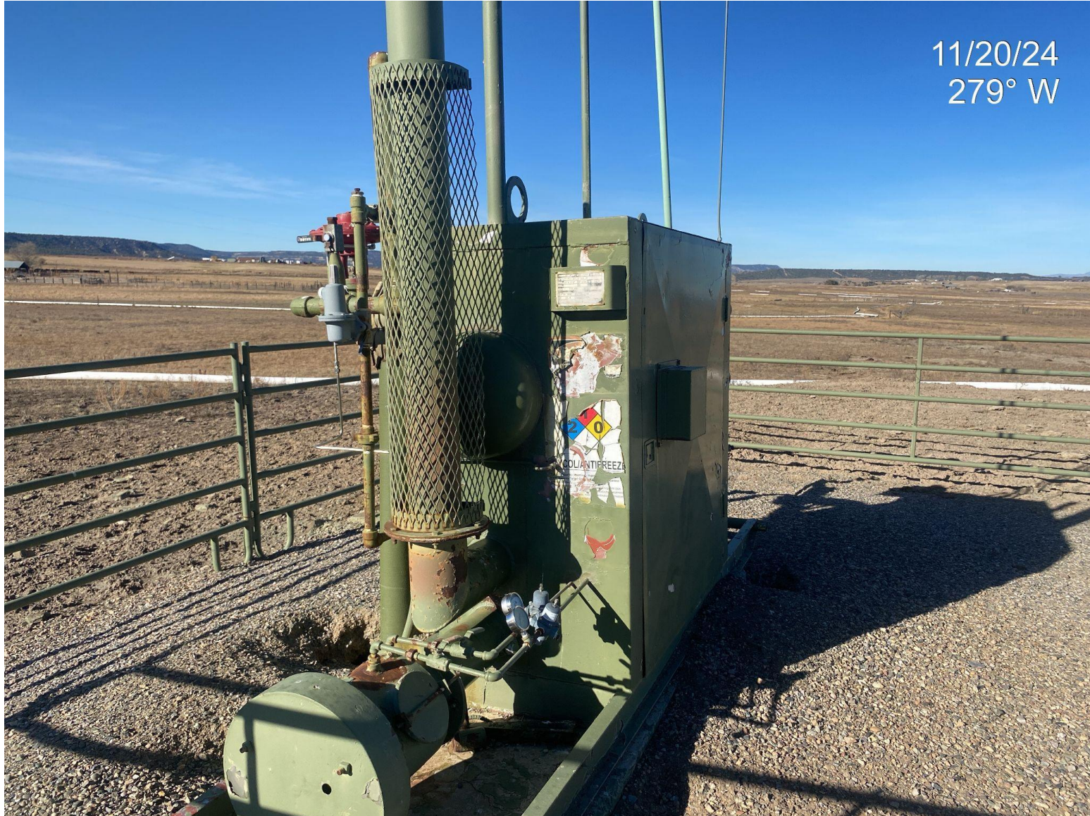
Photo 3. Placard/sign at separator is starting to deteriorate, future maintenance is advised.
