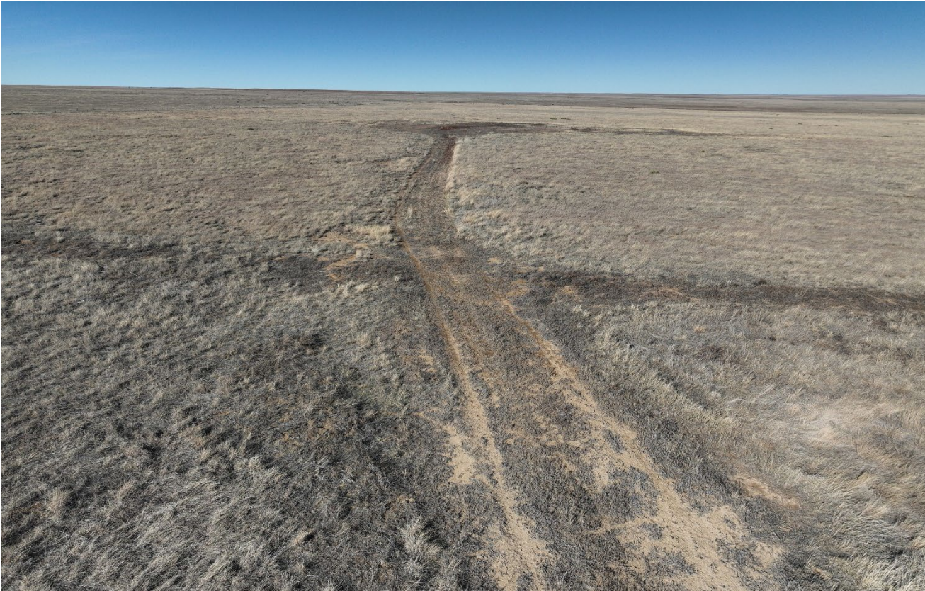
Photo 3. Drone aerial photo facing northeast along the former access road. The perennial vegetation does not appear to be establishing.
