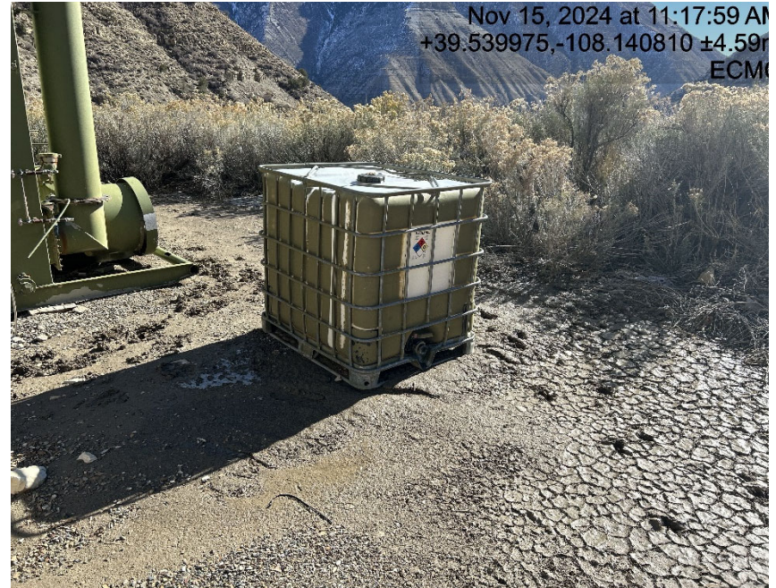
Chemical tank not contained
