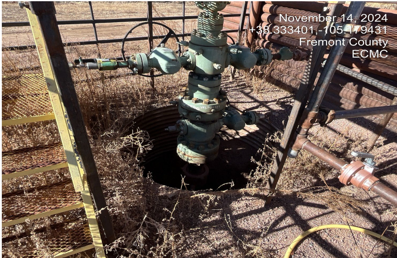
Photo 8. The open cellar at the wellhead needs to be covered or have an escape ramp for critters.
