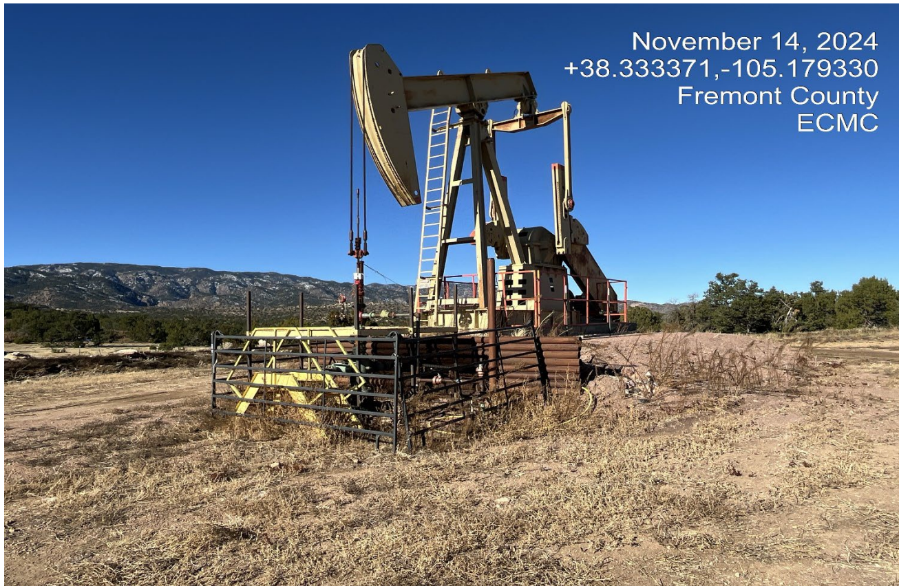
Photo 7. Facing toward the wellhead. The area around the equipment needs to be kept free of dry vegetation and debris.
