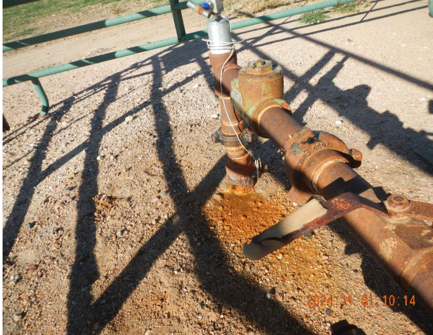
3. Wet area noted around water leg of wellhead.
