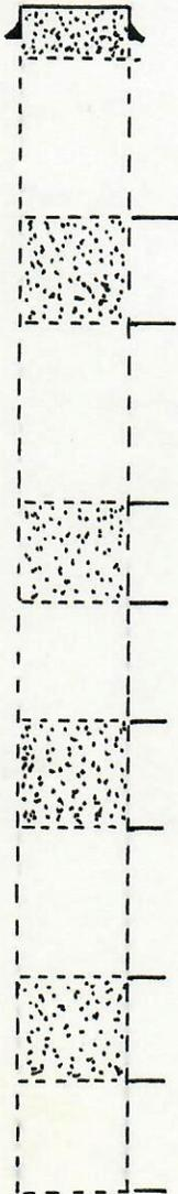
Top of well capped with steel plate welded to casing. Surface casing (55' of 8-5/8") filled with cement and bottom of surface plug at 85' depth. 27 sx. plug
