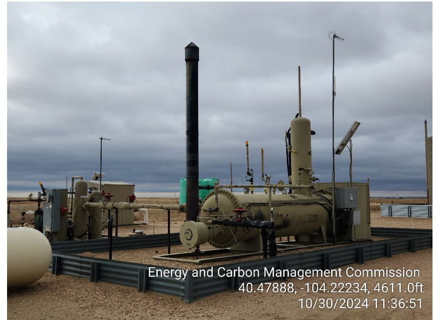
Photo 4 – Separator and VRU
