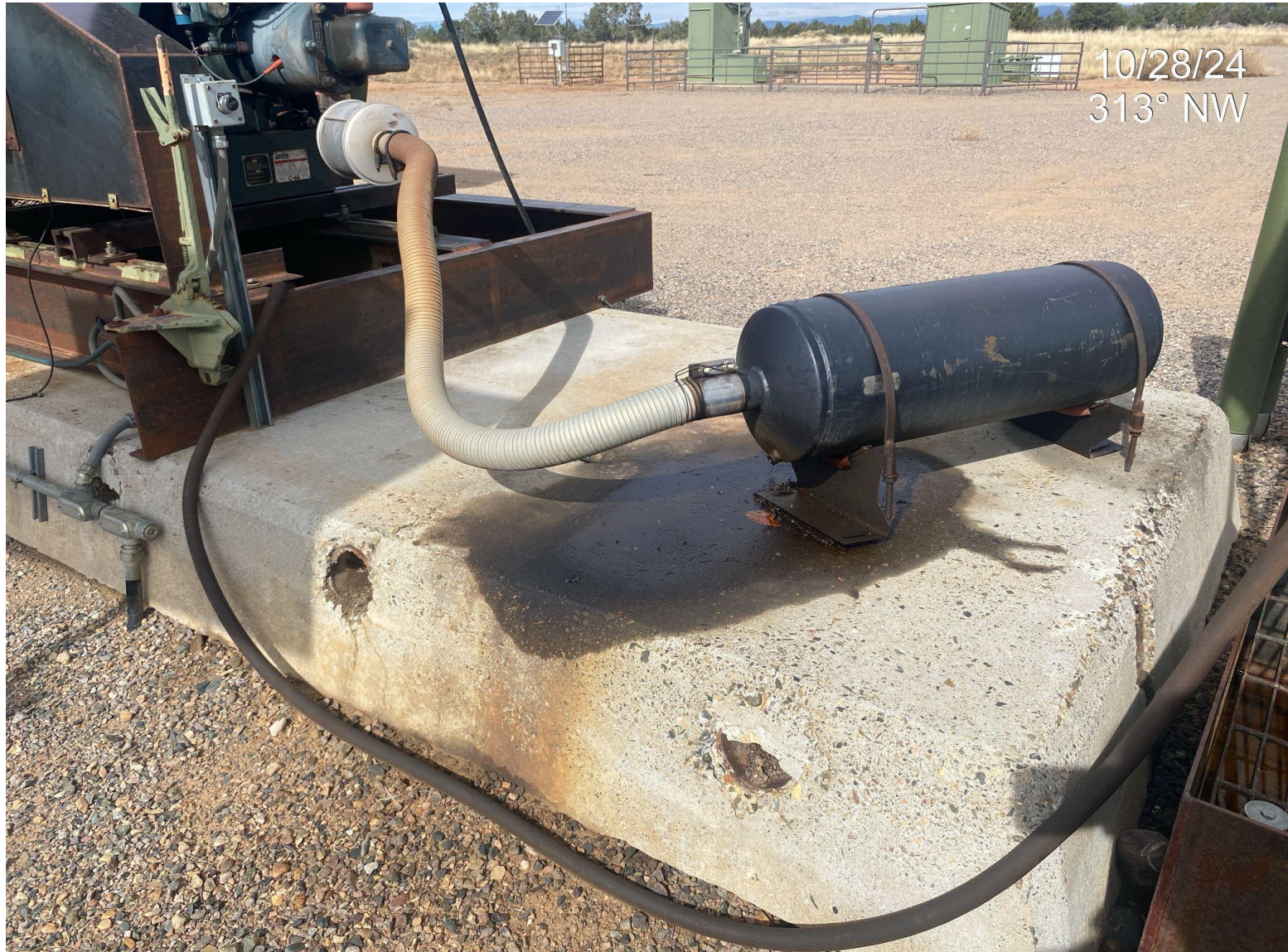
Photo 3. Small spill observed on pump jack pad at muffler.
