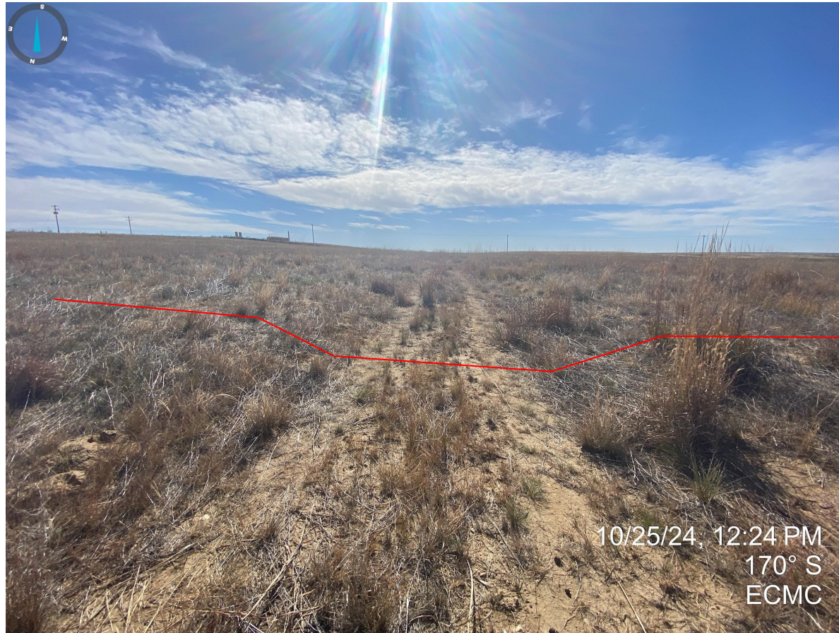
Photo 2. Facing south along the access road. Red line illustrates that portions of the former access road do not appear to have been recontoured.
