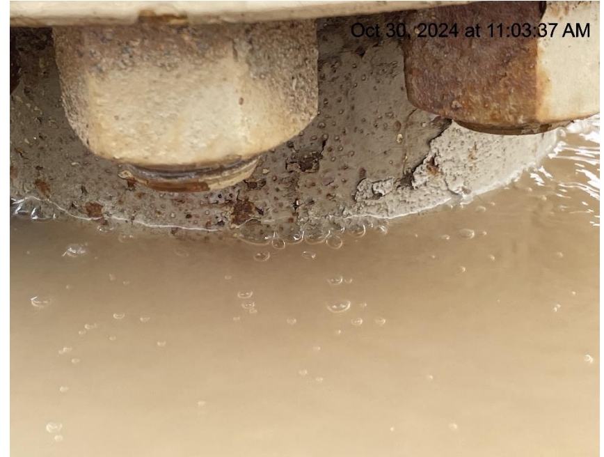
Photo # 8152 Possible wellhead leak/gas bubbling up through water around wellhead (FEDERAL RMV 63-19 well)
