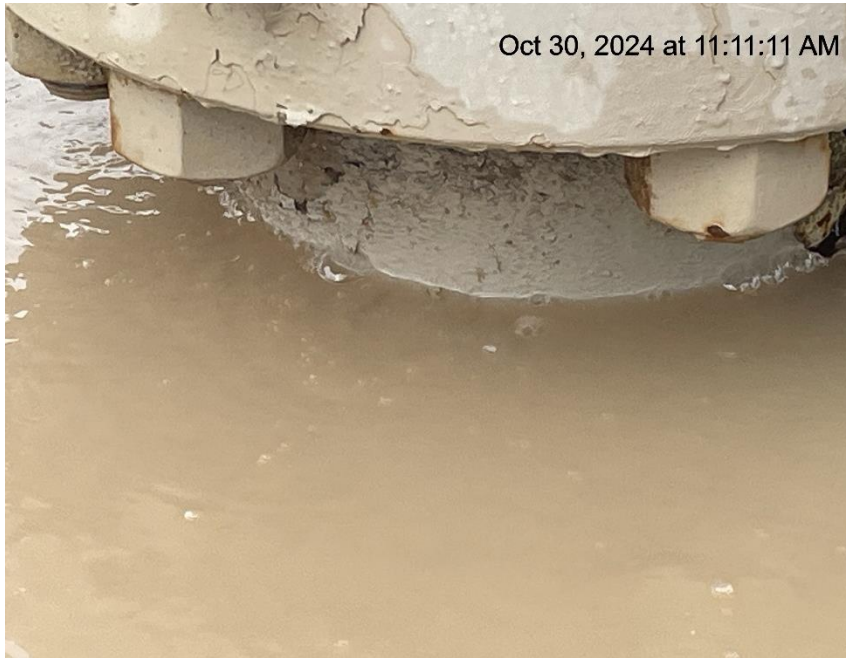
Photo # 8155 Possible wellhead leak/gas bubbling up through water around wellhead (FEDERAL RMV 63-19 well)
