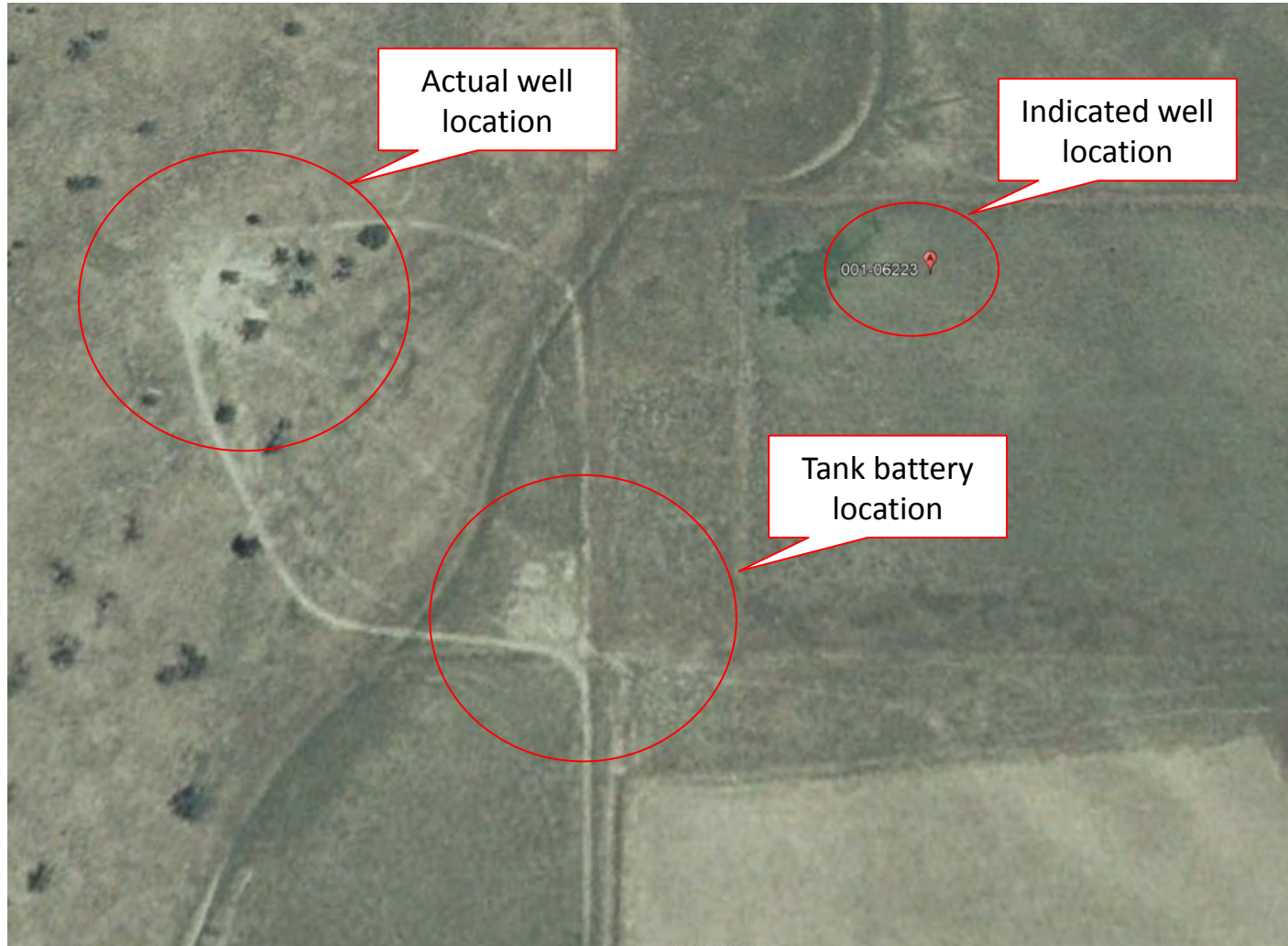
Photo 6. The photo was taken with Google Earth imagery. The image illustrates the indicated lat, long of the well location is incorrect based on the disturbance area and details from Doc #'s 200043160 and 1247886.
