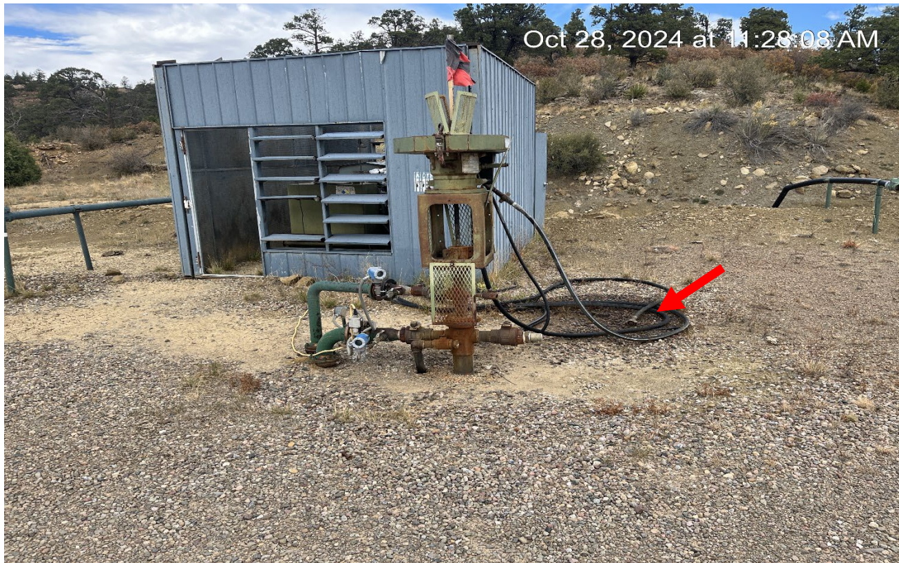
Photo 3. Facing toward the wellhead. There is stained soils at the hose outlet at red arrow.
