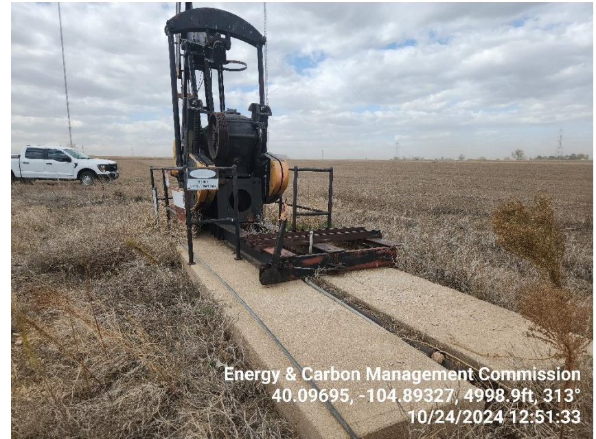
Photo 6 Electric motor has been removed.
