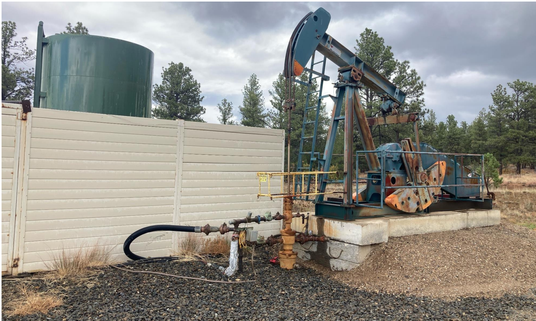
PHOTO 3: WELLHEAD AND EQUIPMENT.
