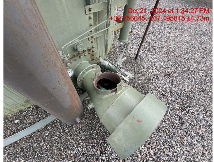
Photo # 7722 Tank heater open to wildlife hazard/ available for entry by wildlife
