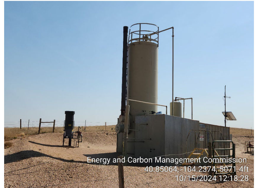
Photo 2 – Heater Treater and ECD
